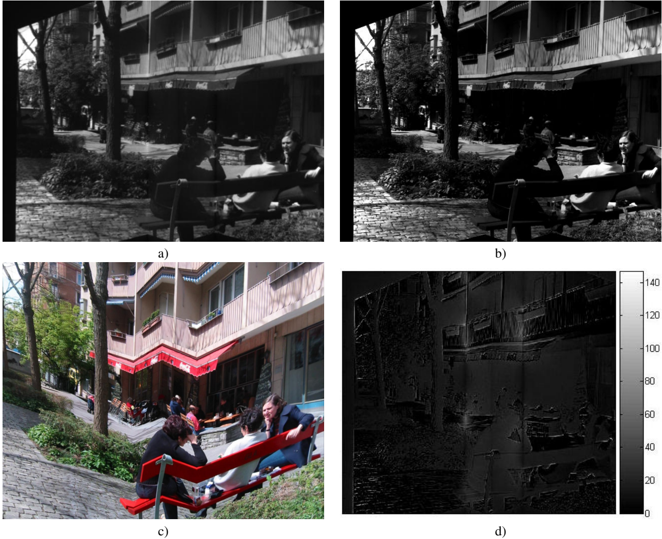
Figure 4. a) An image captured by a camera. b) An image rendered to predict the captured image. c) The projected image that was captured. d) A contrast-enhanced difference image of the captured and predicted images.
