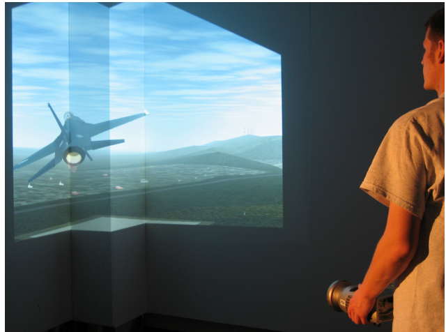
Figure 1. Our tracking process adapts to changes in projector pose, allowing “on the fly” display reconfiguration.
